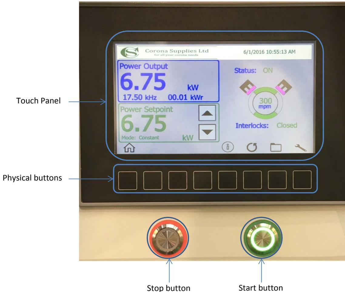
Touch panel – Used to make changes to parameters and show generator information
