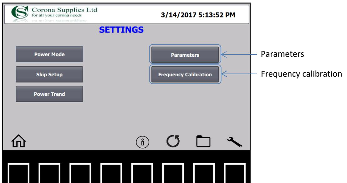
Parameters - Press to enter the supervisor parameters screen where limited machine parameters can be adjusted.
