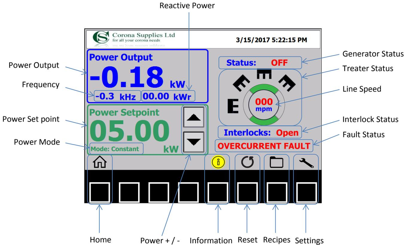
Power output - Indicates the current output power in kW
