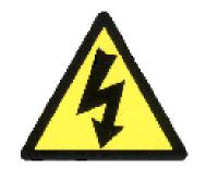
Corona treatment equipment operates at very high voltages ( up to 15000 volts) at electrodes. It is essential that the utmost caution is taken when operation and maintaining equipment, where dangerous voltages are present they are indicated by the hazardous voltage warning label ISO 3864 No. B.3.6. No access is permitted to the area indicated by this symbol <u>UNLESS</u>
