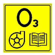
The treatment process produces ozone gas as a by product. It is the customer's responsibility to ensure that the unit is connected to a suitable extraction system and or catalytic converter constructed from corrosion resistant materials.
