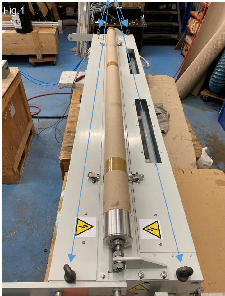
Lifting eyes screwed in to sideframes
